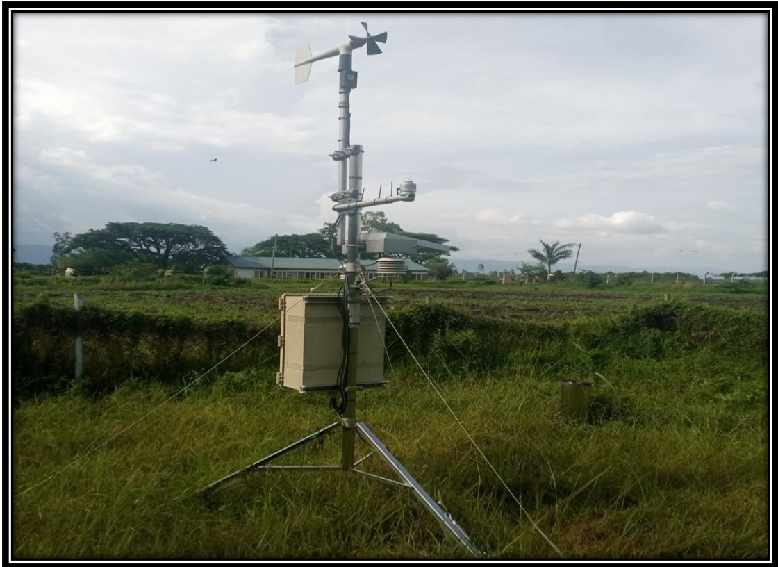
Figure 3.8: Weather station with a thermometer used to measure temperature
