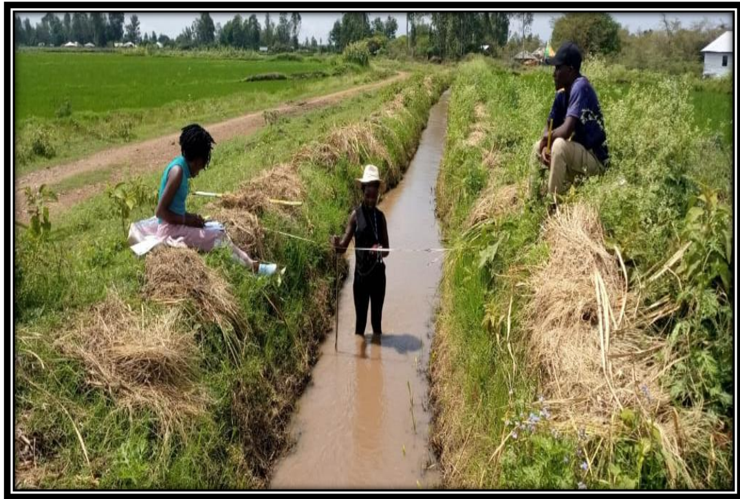
Figure 3.6: Discharge measurement in the earthen canal
