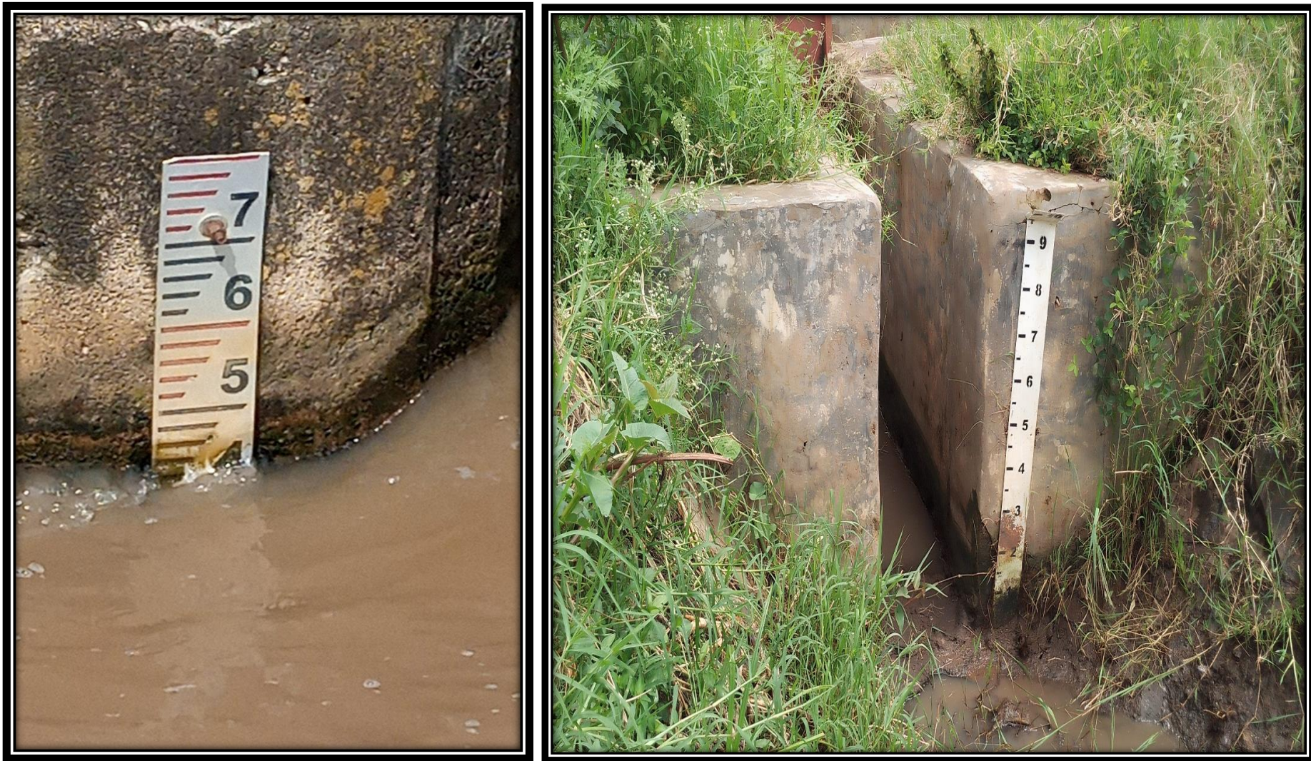
Figure 3.5 Staff gauge aids in measuring the depth of water in the canal
