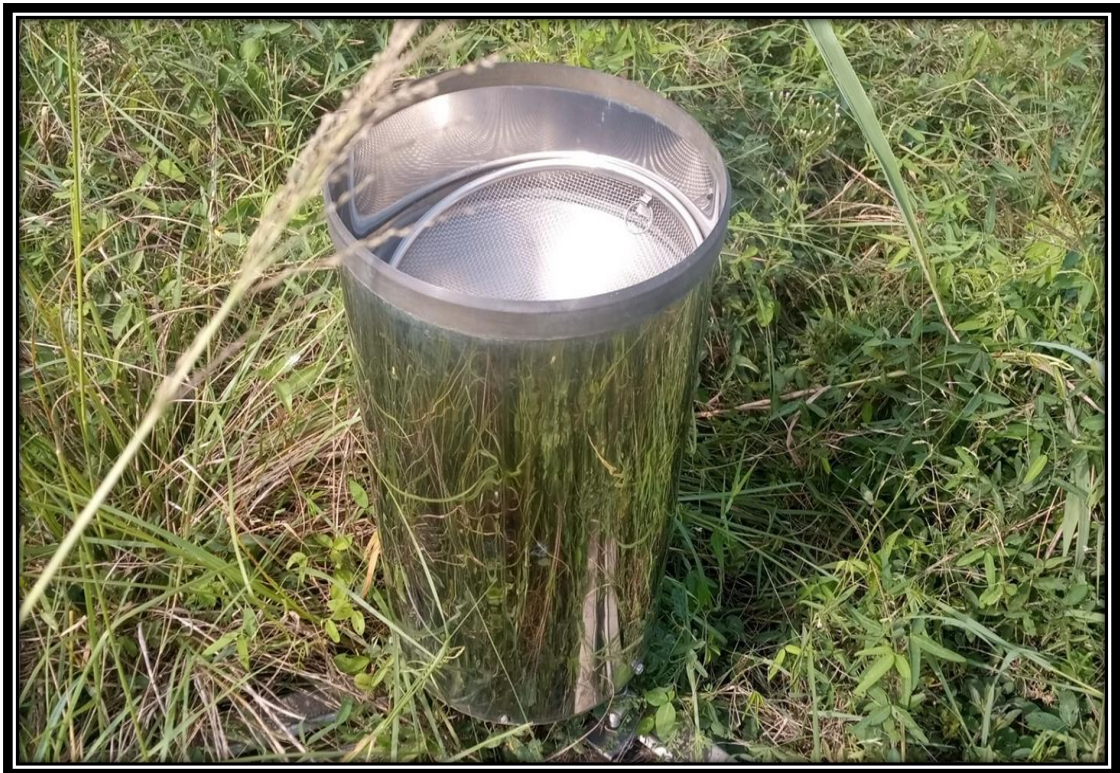
Figure 3.9: Rain gauge used to measure rainfall
