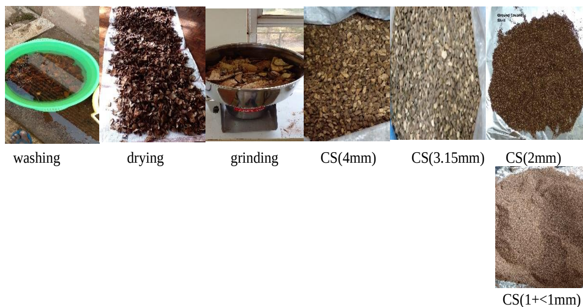
Figure 3-5 Reinforcement preparation (washed, dried, ground and sorted to different sizes)
