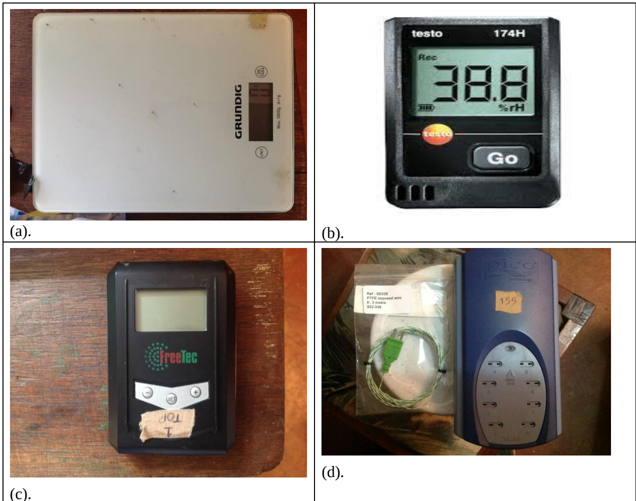
(a)-Digital measuring scale (weighing cowpea), (b)-Testo Data Logger (Temperature and Relative Humidity capture), (c)-FreeTec Data logger (Temperature and R.H. capturing),(d)- Pico TC-08 Thermocouple data loggers and SE 000 PTFE) type K Thermocouple (Temperature capturing and data storage).
