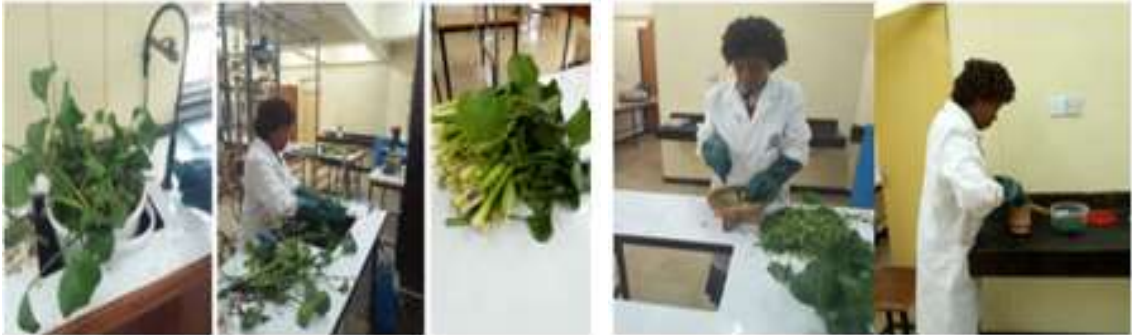
Figure 3. 3: Washing, cutting, and mashing of water hyacinth to be ready for digestion
