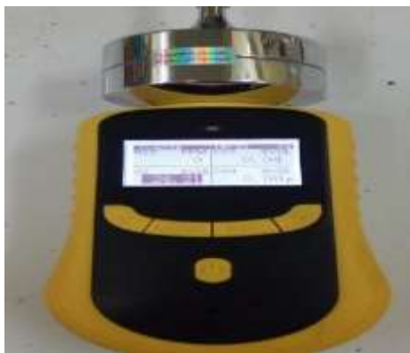
Figure 3. 10: A multi-gas detector used for biogas analysis
