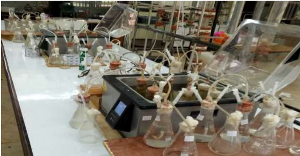
Figure 3. 15: Illustration of the experimental setup of anaerobic batch fermenter of FW and WH
