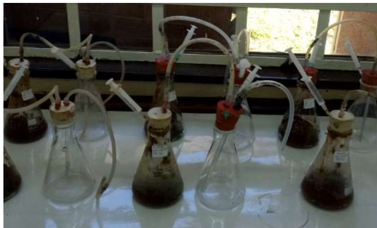
Figure 3. 6: Prepared digesters with cocks, rubber pipers, non-return valves, and syringe
