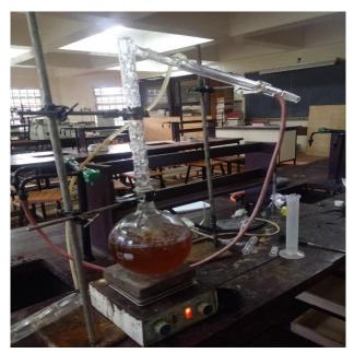
Figure 3.3 Recovering methanol from WCO, methane, and NaOH involves heating, stirring, and collecting condensed vapor.
