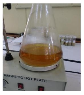
Figure 3.8: Evaporation of Water from Biodiesel Utilizing Vaporization technique
