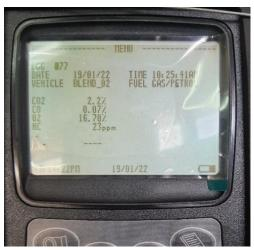
Figure 3.14: Gas detector displaying levels of CO<sub>2</sub>, CO, O<sub>2</sub> and HC
