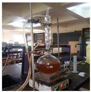
Figure 3.2: WCO, methanol, and NaOH are heated and stirred, with evaporating methanol condensed back into liquid.
