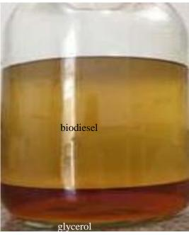
Figure 3.4: After 12 hours of cooling, glycerol and biodiesel undergo sedimentation, revealing insights into their separation behavior.
