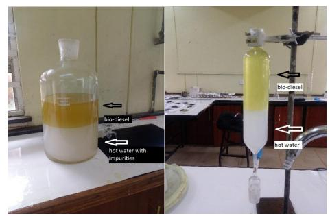
Figure 3.7: Washing biodiesel in hot water results in a purer end product, highlighting its importance in improving overall synthesis quality.
