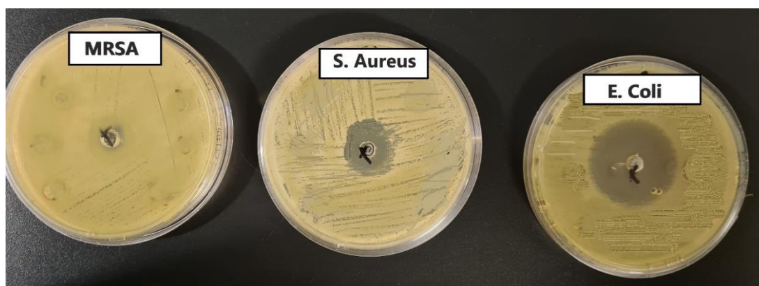
Figure 4:17. Test Results of Agar Well Diffusion of Silver Nanoparticles against MRSA , E. coli and S. aureus
