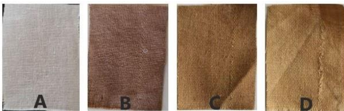
Figure 4:4. 100 % Cotton fabrics. A - Untreated, B - Treated with AgNps before Washing, B - Treated with AgNps after 10 Washes and C - Treated with AgNps after 20 Washes
