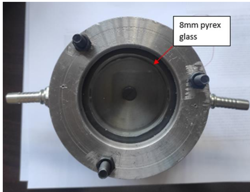
Figure A1: Cross filtration setup top view
