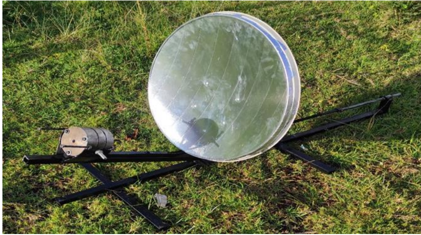
Figure A3: Manual solar tracking with parabolic dish concentrator and cross filtration set-up.
