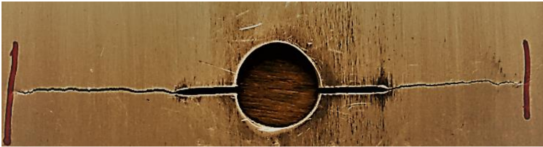
Figure 4.16: Crack path for Al alloy 7075-O.
