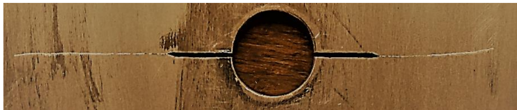
Figure 4.17: Crack path for Al alloy 7075-T6.
