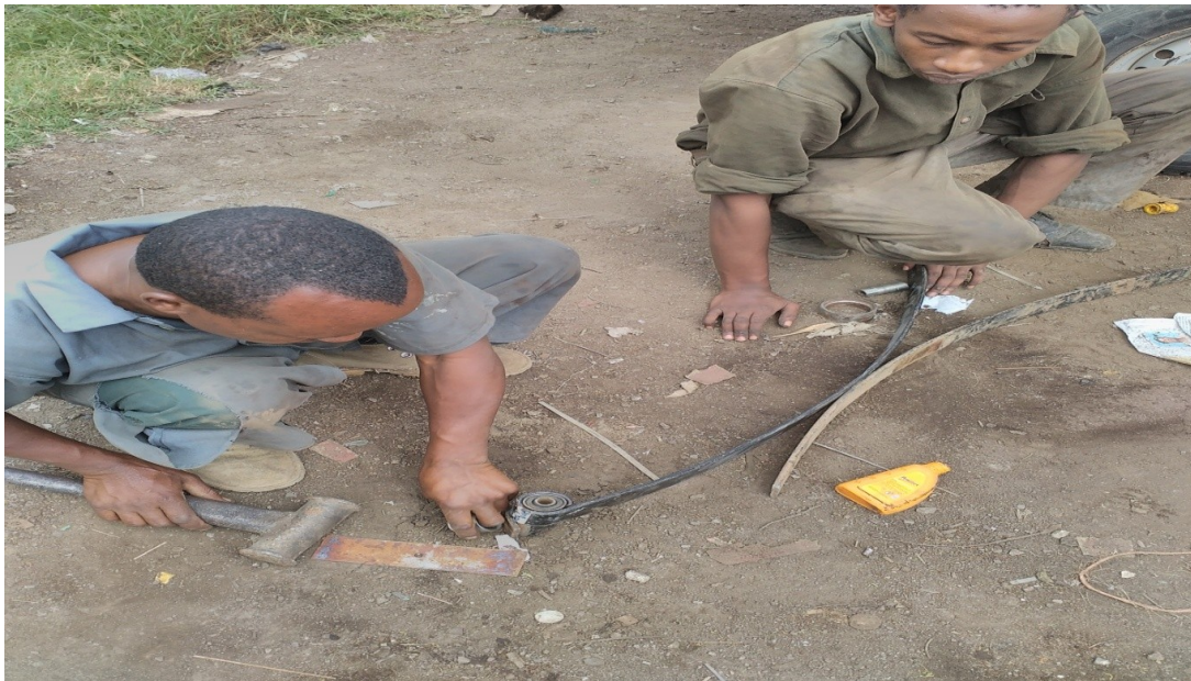
Jua Kali automotive engineers in outer estate fixing a truck's suspension system; these are skills mostly learned through apprenticeship or from technical institutions. However more and
