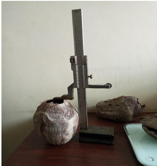
Figure A-4 Weight and length measurement of immature coconut husk waste after drying
