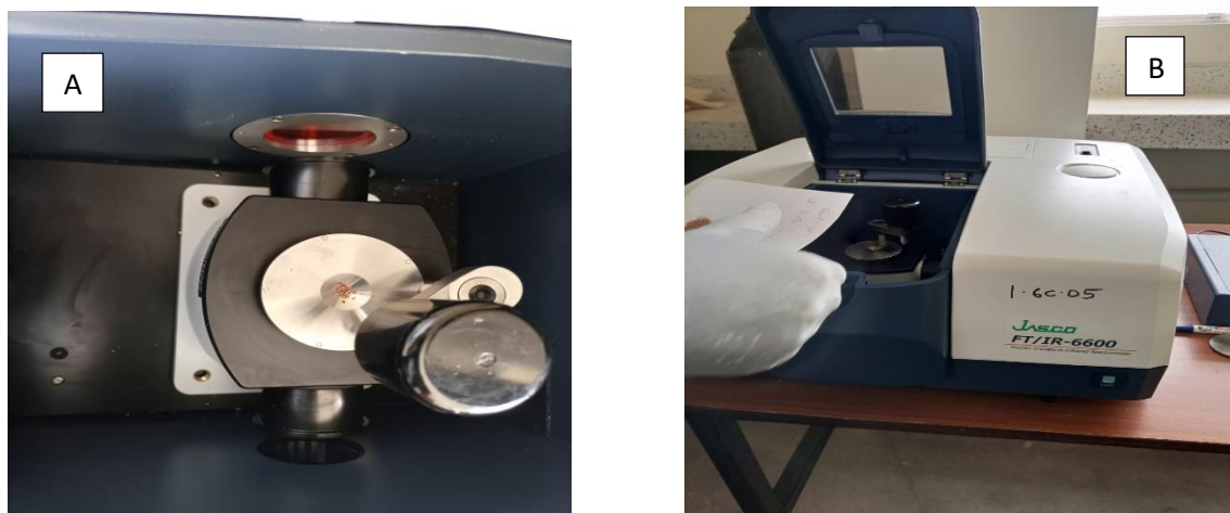
Figure 3-6 Infrared spectroscopy of coconut fibers using Jasco FTIR
