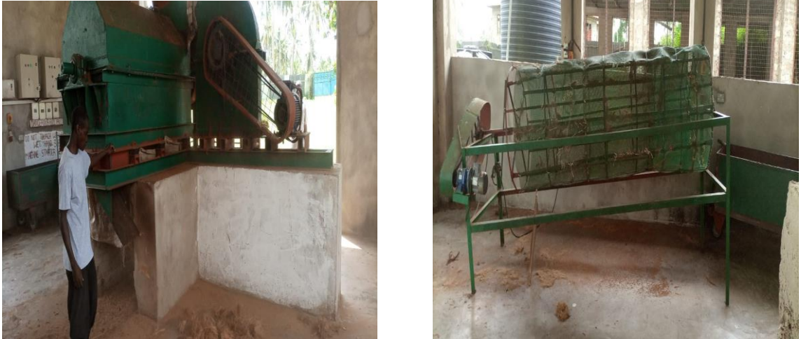
Figure 3-2 Decorticator and fiber screener used for fiber extraction
