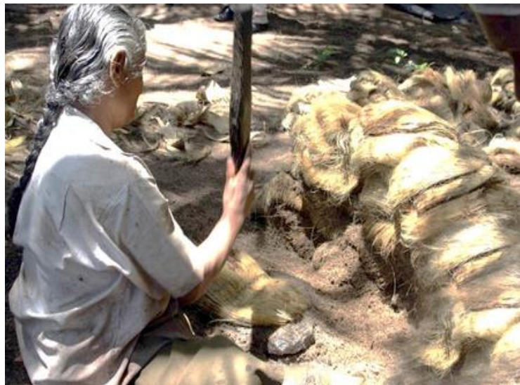
Figure 2-1 Manual defibering of retted husk.
