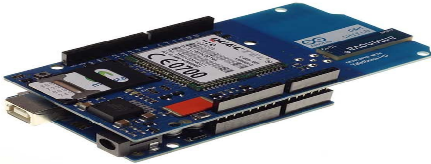
Figure 2.4: Arduino communication shield
