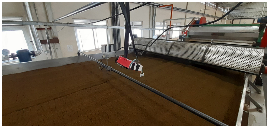
Figure 8. Application of Raspberry Pi 3 Model B+ with the Pi camera for taking pictures during the fermentation of black tea in the Sisibo Tea Factory, Kenya.
