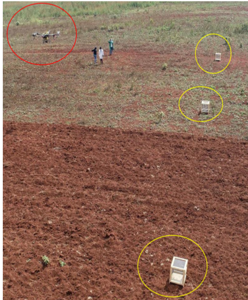
Figure 3. Wire mesh cages (objects arranged within the yellow circle) with live locusts arranged parallel to the drone flight path (object within the red circle).
