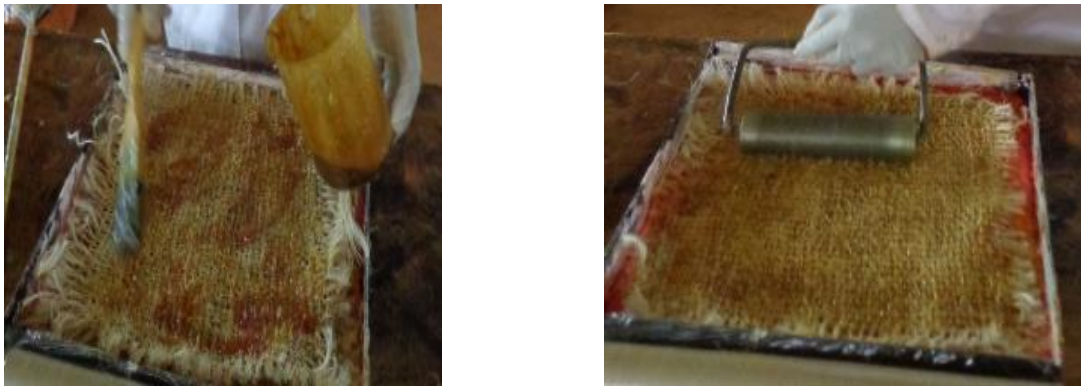
Figure 3.6: Application and squeezing the matrix into the fibres
