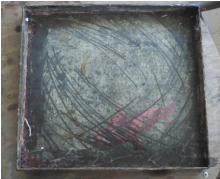
Figure 3.5: A mould measuring 310 x 310 x 10 mm
