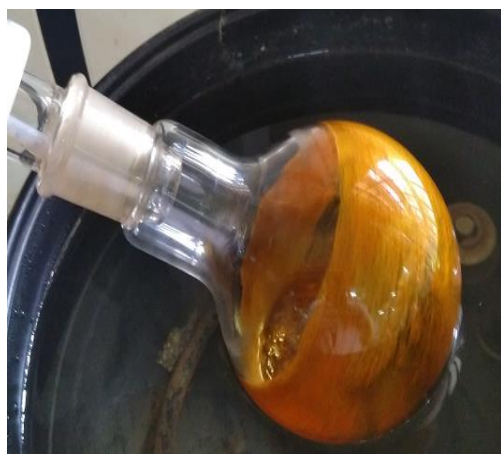
Figure 4.9: Removal of the excess solvent from embelin crude sample
