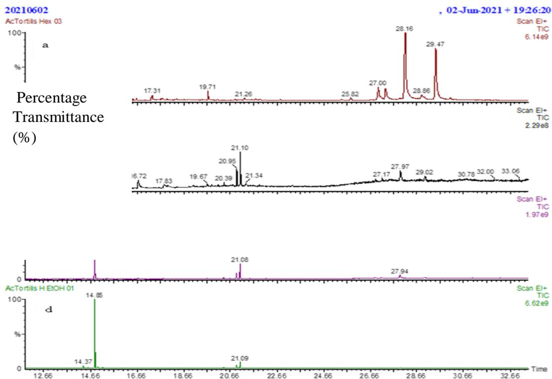
**Figure 17:** GC chromatogram for a; hexane, b; ethyl acetate, c; acetone and d; ethanol extract
