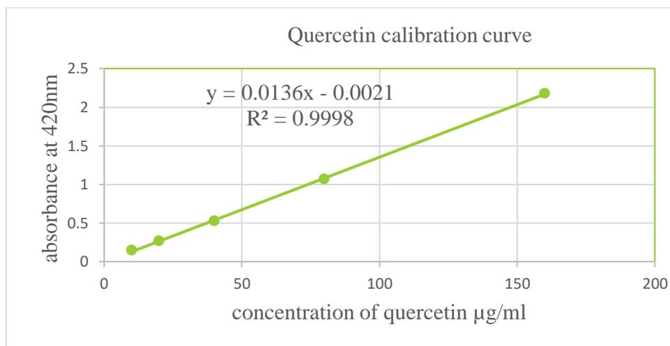
**Figure 13:** Standard curve for determination of TFC
