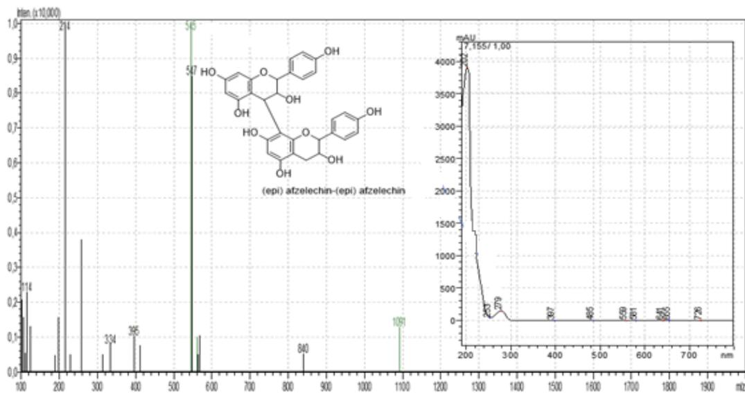
**Figure 22:** MS spectra, PDA spectra and chemical structure of (epi) afzelechin- (epi) afzelechin
