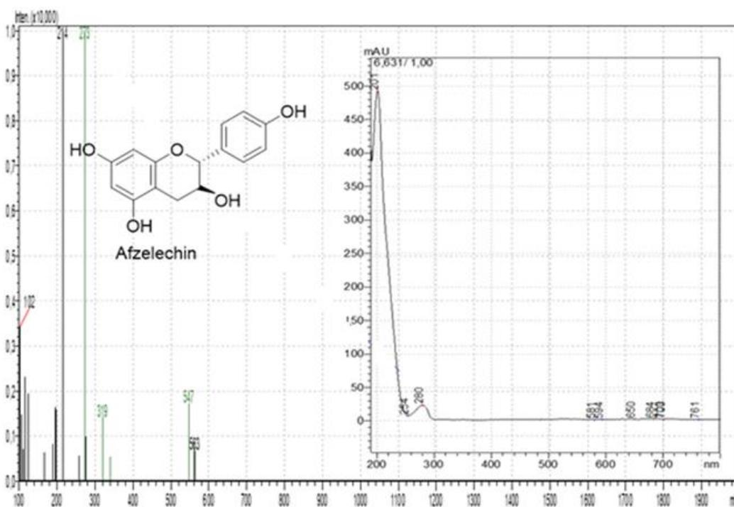
Figure 25: Mass spectra, PDA spectra and chemical structure of Afzelechin
