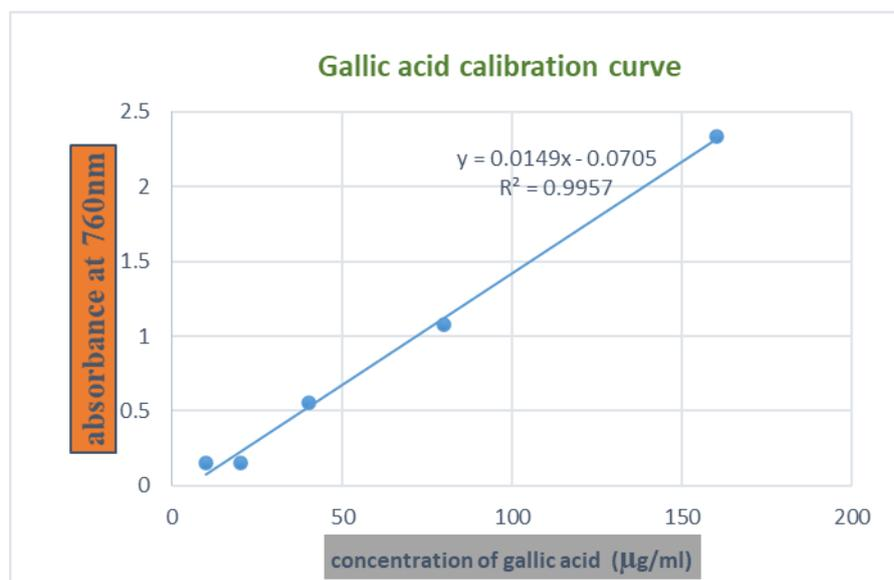
**Figure 12:** Standard calibration curve for determination of TPC
