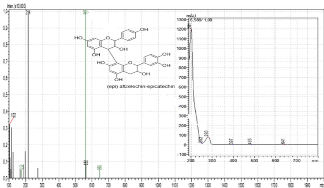
**Figure 21:** MS spectra, PDA spectra and chemical structure of (epi)afzelechin-epicatechin
