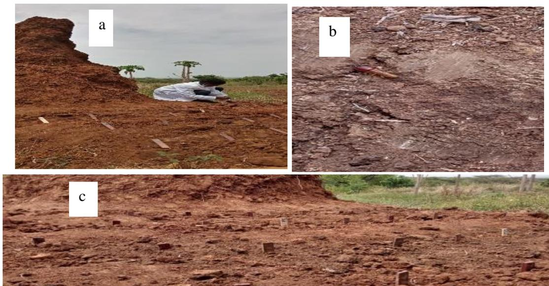
**Figure 10:** (a): Arrangements of wood blocks around termite nest, (b): *Macrotermes natalensis* and (c): buried wood block arranged so that the distance between each block is 20 cm and 30 cm from the termite nest.
