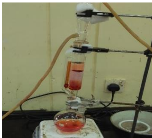
Appendix 2: Soxhlet apparatus in solvent extraction of B. vulgaris peels and pomace and crude extract.
