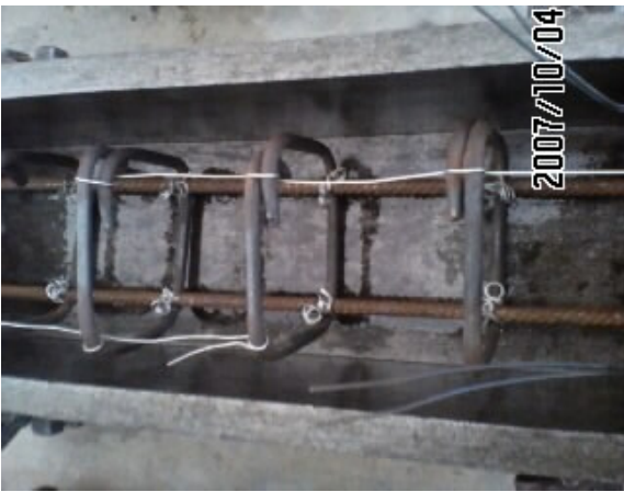
(c) Short beam stirrup-rebar's cage
