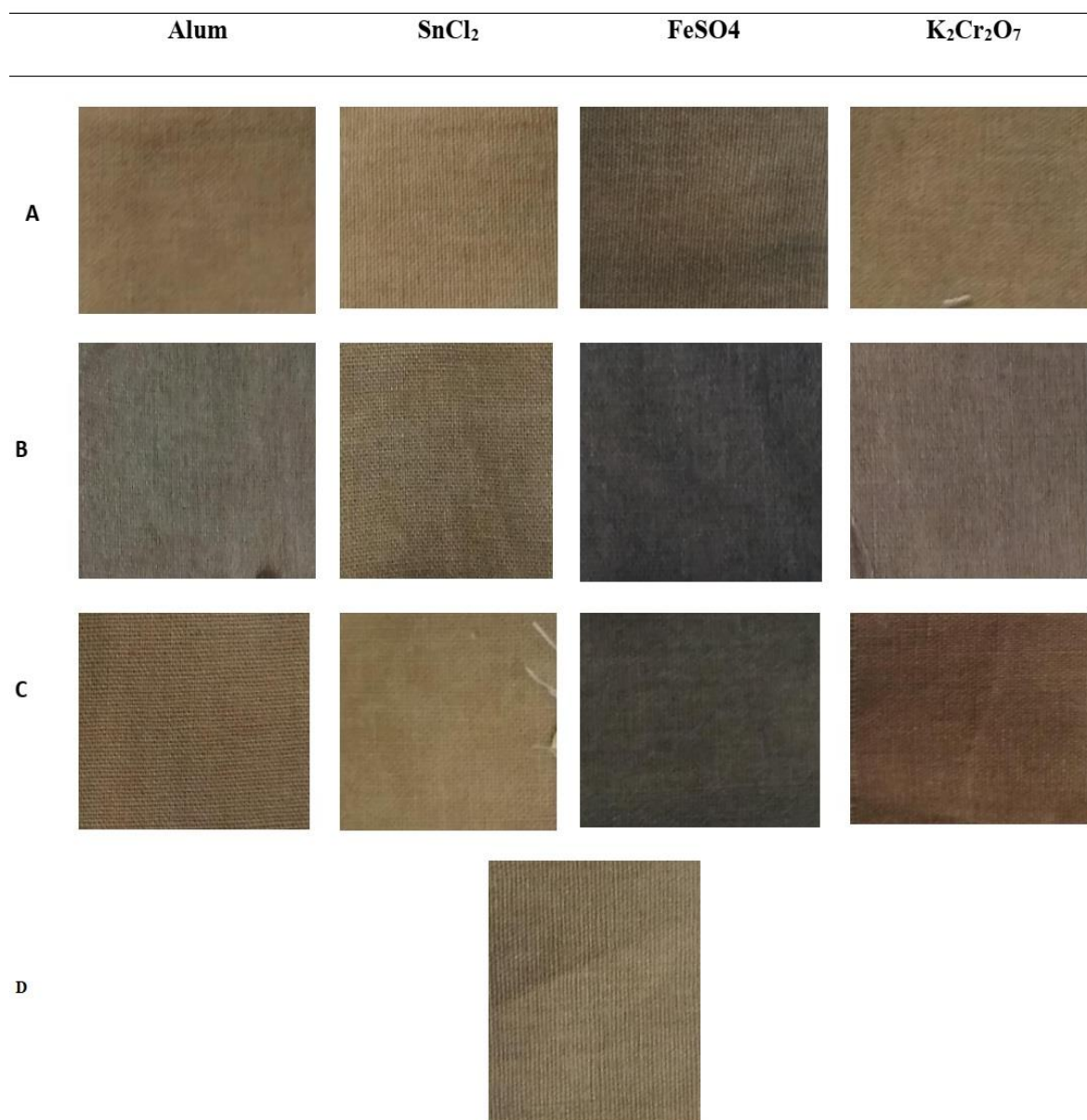
Figure 4.13: Dyed fabric in combination with different mordants and mordanting techniques
