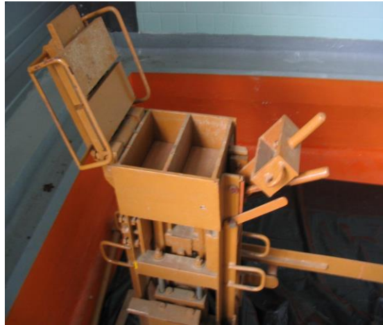
Fig. 3.3 “Balram” Block press “Artifact gmbH”
