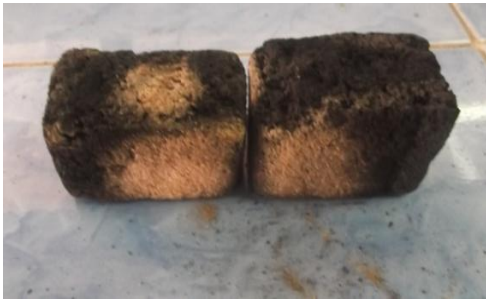
Fig. 12. Briquettes with clay binder retained shape on burning
