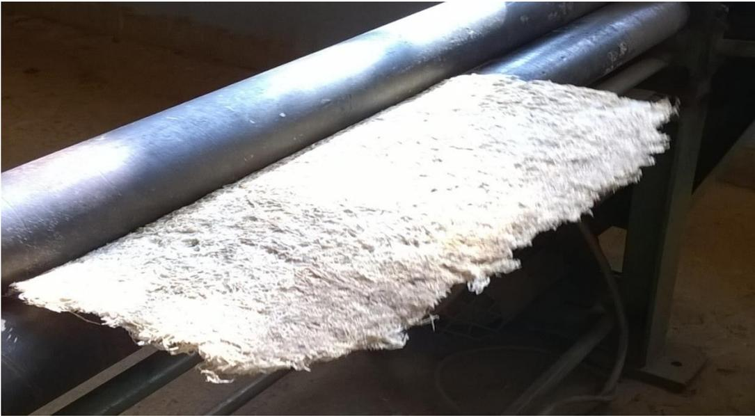
**Figure 16: Consolidating the nonwoven structure from *luffa cylindrica* fibres**
