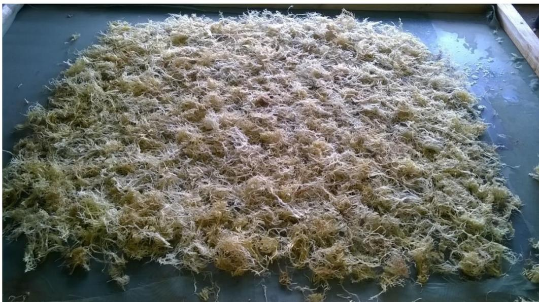
**Figure 14: The random dry-laid web from *luffa cylindrica* fibres**
