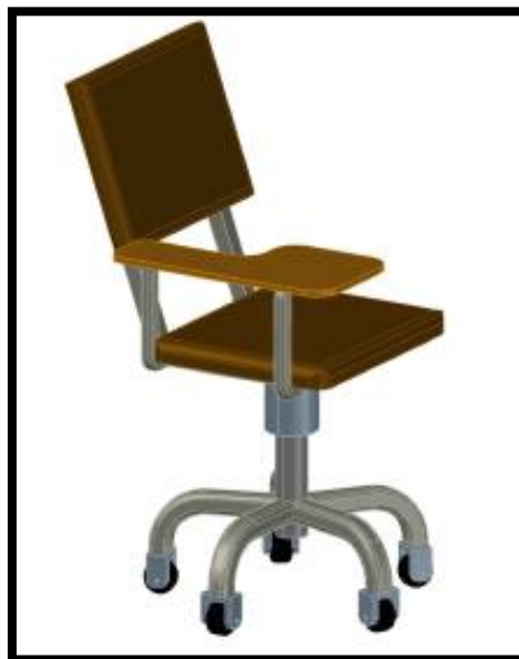
Figure 4.2b: Complete model of the proposed adjustable students' desktop-chair.
