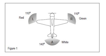
(c) a white light projected above and below the horizontal plane rearward through angle of coverage A.
