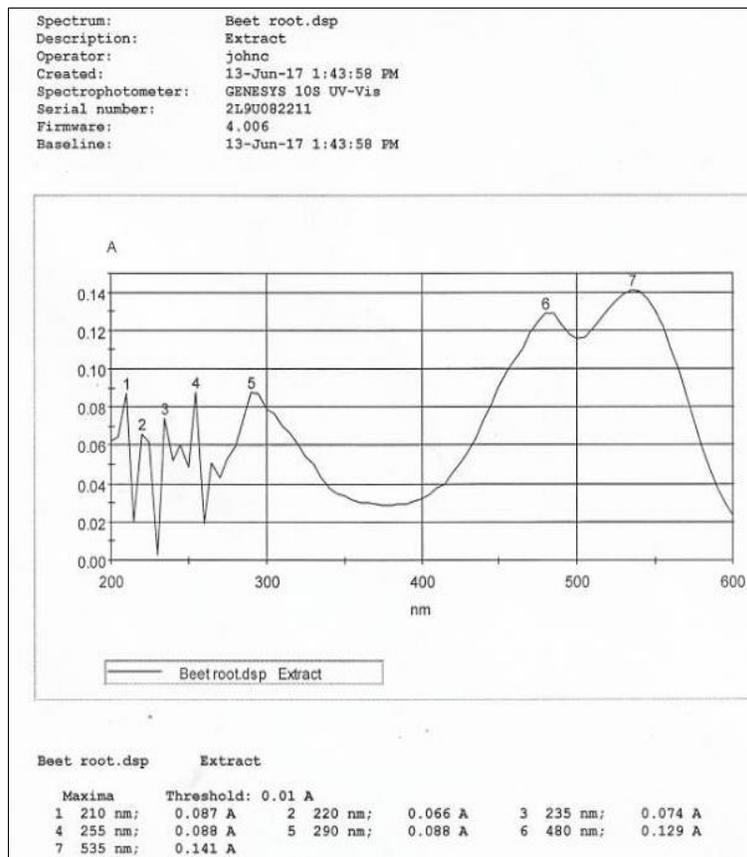
**Fig. 3:** Absorption spectrum for beet root extract
