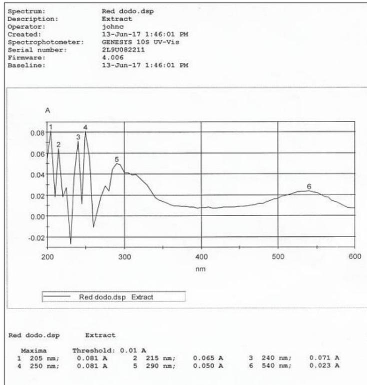
Fig 6: Absorption spectrum for red dodo extract
