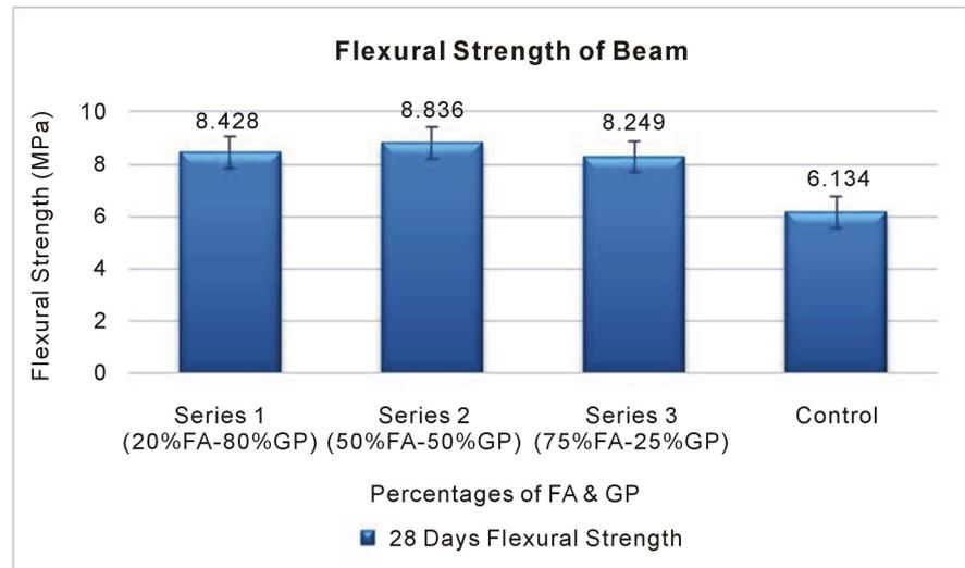
**Figure 4.** Flexural Strength of RRPC Beam containing of FA and GP at 28 days curing ages.
