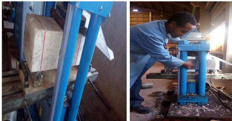
**Figure 5.** Flexural strength test in the laboratory.
