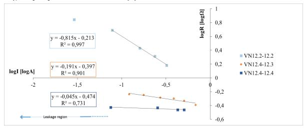
Figure 13. Results of four electrode–four contact measurement. In the leakage region the relation is not according to V=C·I<sup>β</sup>.
