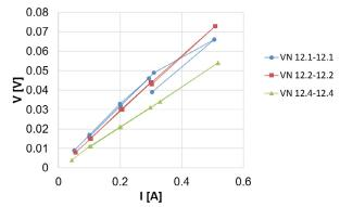
**Figure 9.** Four-point measurement of two hanging stainless steel yarns using different weights – 100 g.
