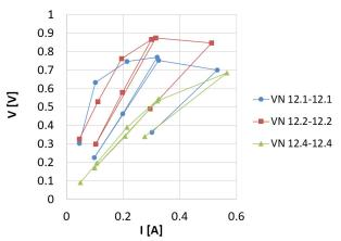
Figure 7. Four-point measurement of two hanging stainless steel yarns using different weights  $-2\,\mathrm{g}$ .
