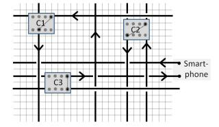
**Figure 2.** A woven circuit electrically connecting a smart phone to the components C1, C2, and C3.
