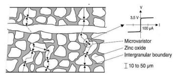
Figure 11. Schematic explaining a commercial metal oxide varistor based on ZnO [11].
