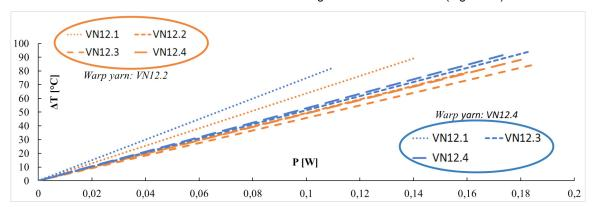
**Figure 14.** Similar  $\Delta T$ —P curves of different electro-conductive (EC) contacts of same plain woven fabrics. Two curves diverge because the EC yarns are thinner and conduction to the adjacent insulating yarns is lower. a > 0.0021 and all  $R^2 > 0.98$ .
