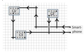
Figure 3. The resulting electro-conductive path.
