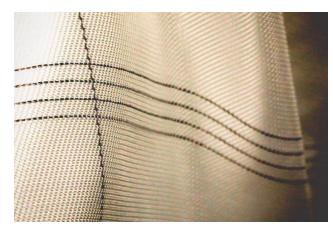
**Figure 1.** A hybrid woven fabric with stainless steel and polyester yarn in a 3/1 twill pattern.
