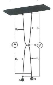
Figure 4. Setup to study the contact between two electro-conductive yarns [10].
