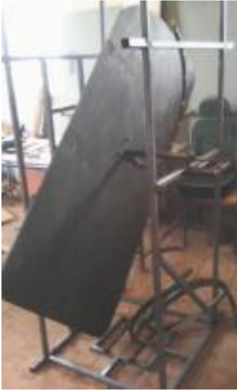
Figure 3.13 (a): turbine 'A' reinforced with plywood.
