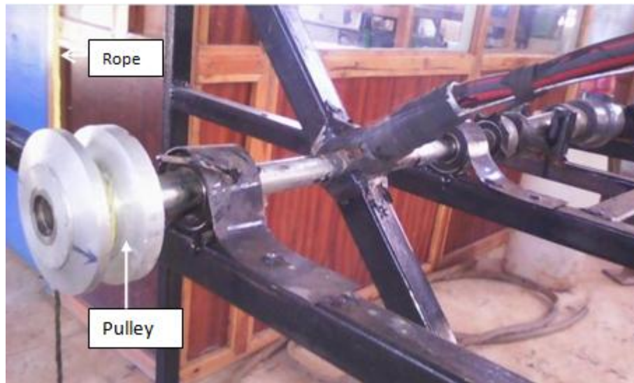
Figure 4.4: Picture of a pulley fitted to a turbine's output shaft
