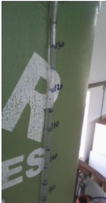
Figure 4.6 (a): Calibrated tank for measuring volume drop
