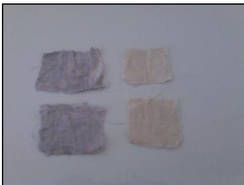
Fig. 2a: Fabric pieces dyed violet in PDB inoculated with Fusarium oxysporum on the left. Controls on the right.
