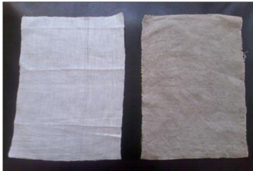
Fig. 2e: Cotton fabric dyed in PDB inoculated with Hormoconisresinae on the right. Control on the left.
