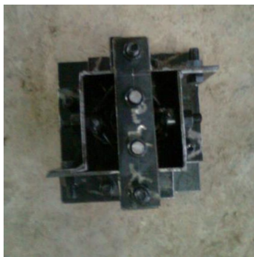
Figure 3.23: Illustration of connector cube mould assembly; side mould, top mould base plate and hooked nuts
