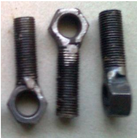
Figure 3.10: Modified nuts with studs for slab panel assembly
