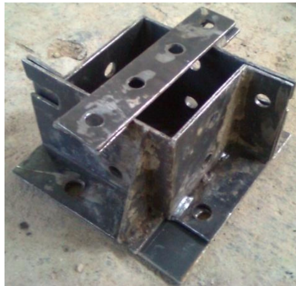
Figure 3.1213: 3D visualization of the connector cube mould
