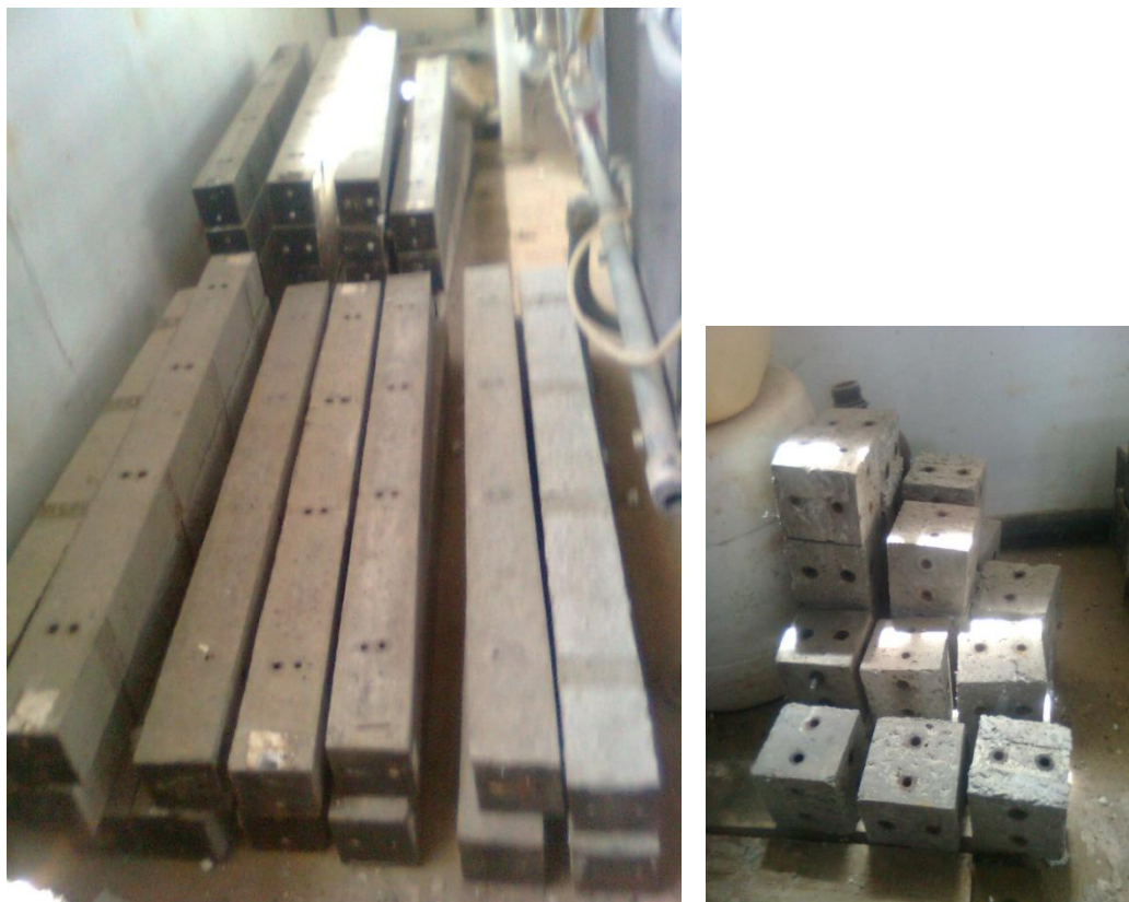
Figure 3.30: Beams/columns and the connector cubes stacked
