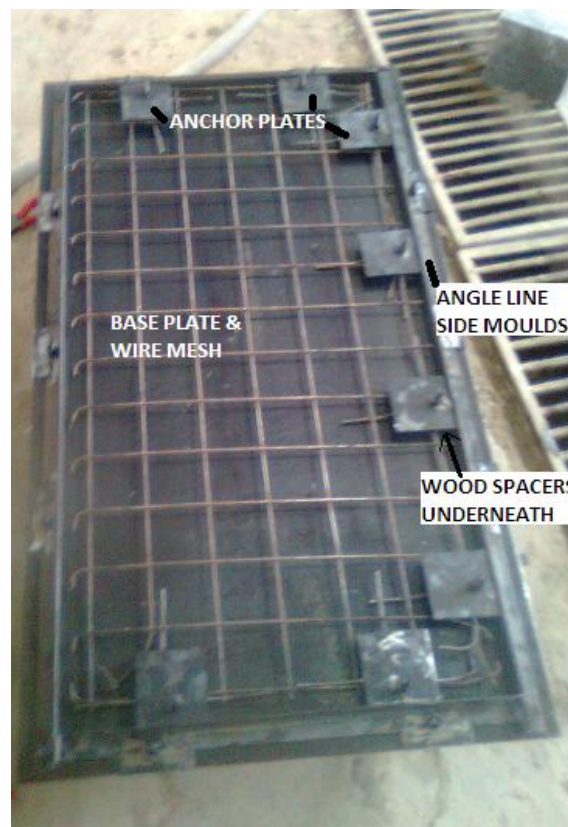
Figure 3.25: Wooden spacers for the slab panels
