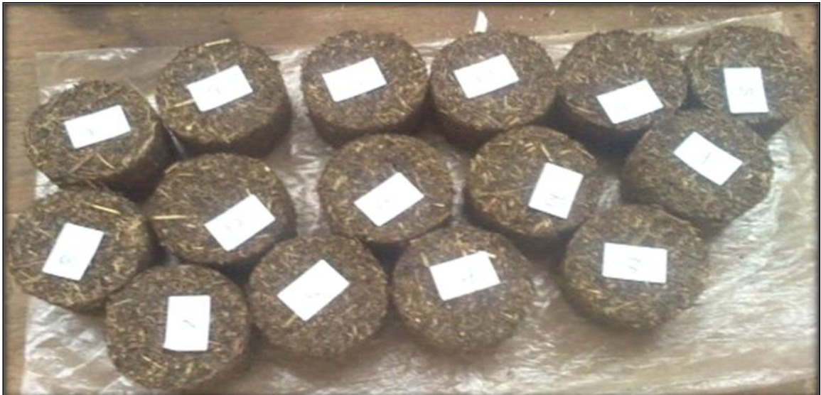
Plate 4.1. TRZE Pellets produced at 20.68bars pressure load.
