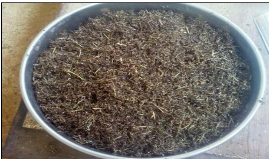
Plate 3.4. Milled TRZE evenly mixed with 15% cane molasses binder
