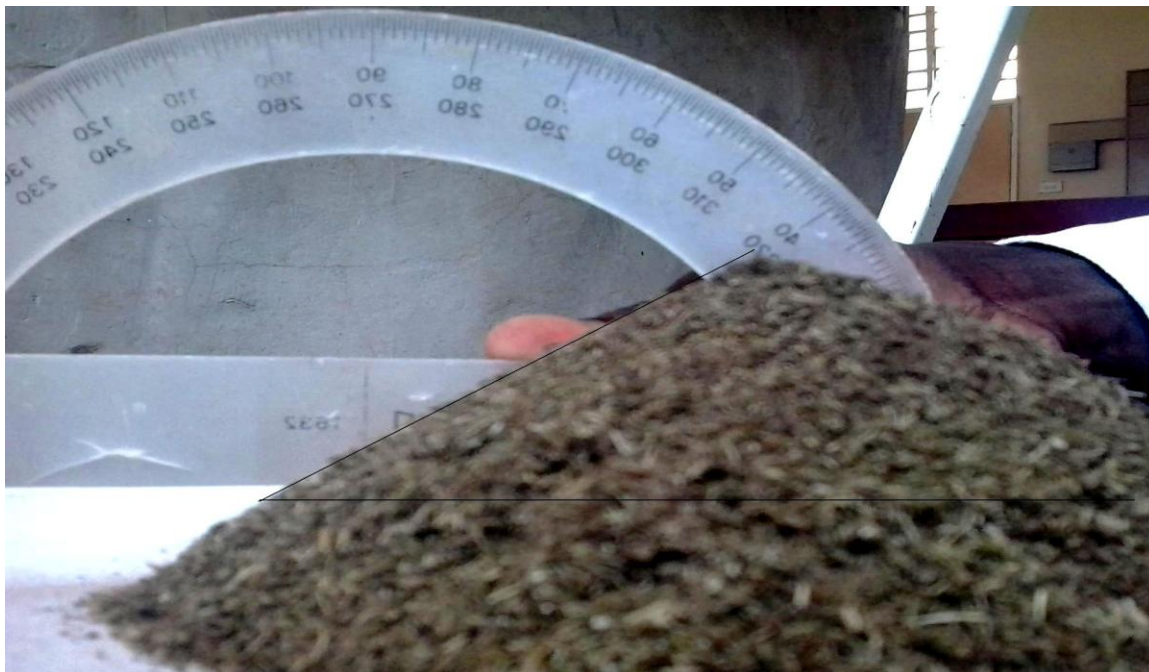
Plate 3.3. Measuring repose angle of 0.6mm particle size.
