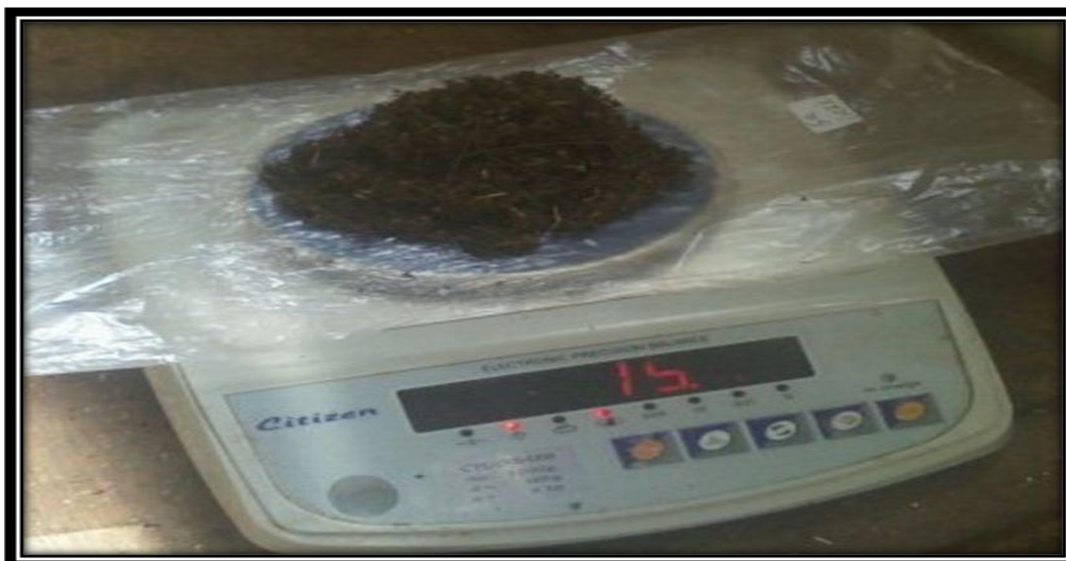
Plat 3.5. Weighing 15.0g of milled TRZE for pellet making
