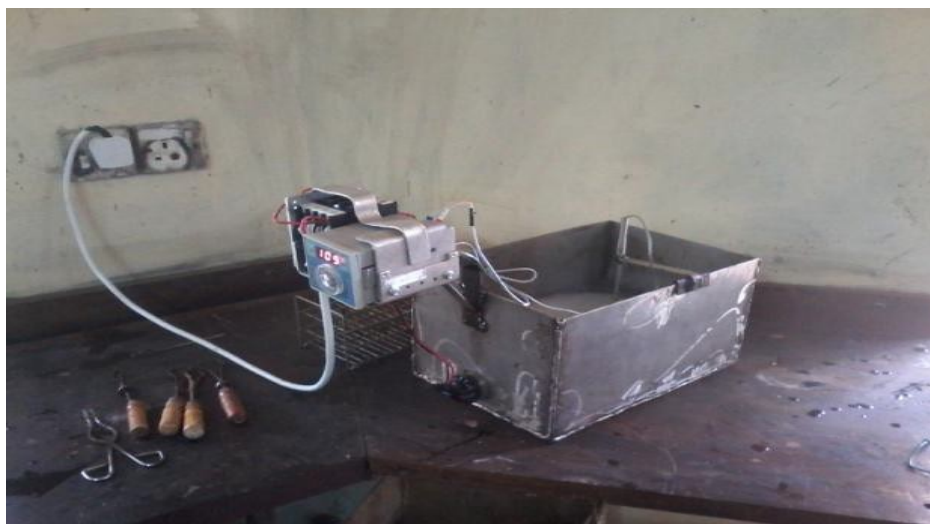
Image 0.3 Fabricated Oil Bath
