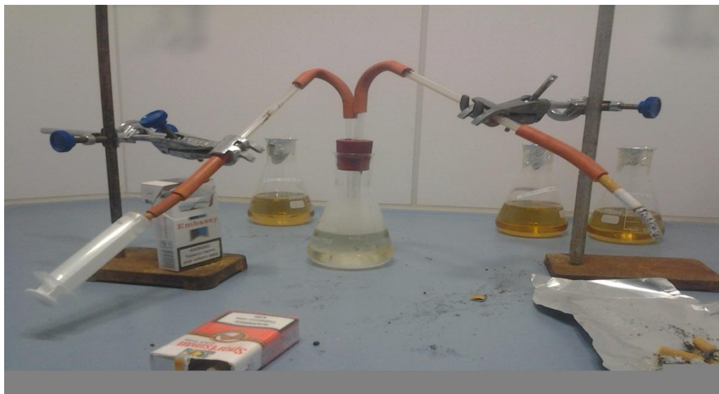
Figure 3.1: The Apparatus Set Up for Cigarette Smoking in the Laboratory
