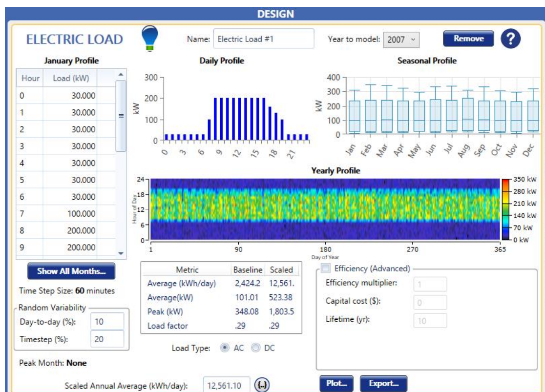
Figure 3.5: load profile of Moi International Airport
