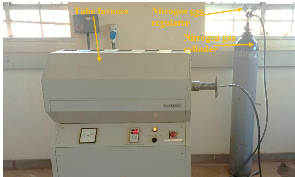
Plate 3.3: Modified tube furnace to torrefaction equipment
