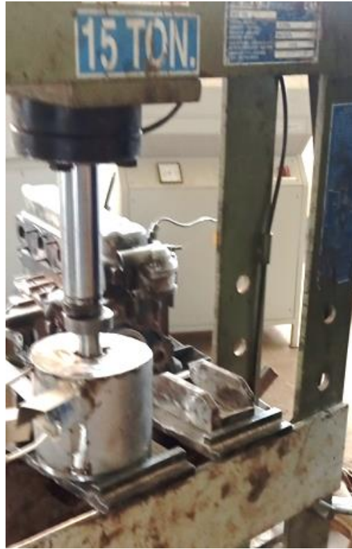
Figure 4.3: Hydraulic press and heated mould in operation
