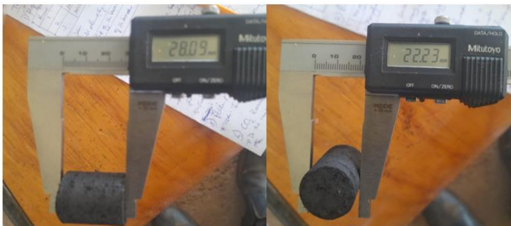
Plate 3.4: Measuring pellet dimensions
