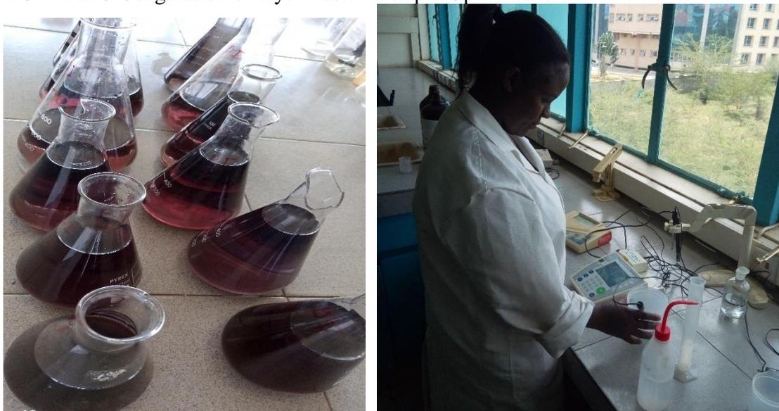
B.3.2: PaFC Coagulation of Dye Wastewater-Dosage Optimization
