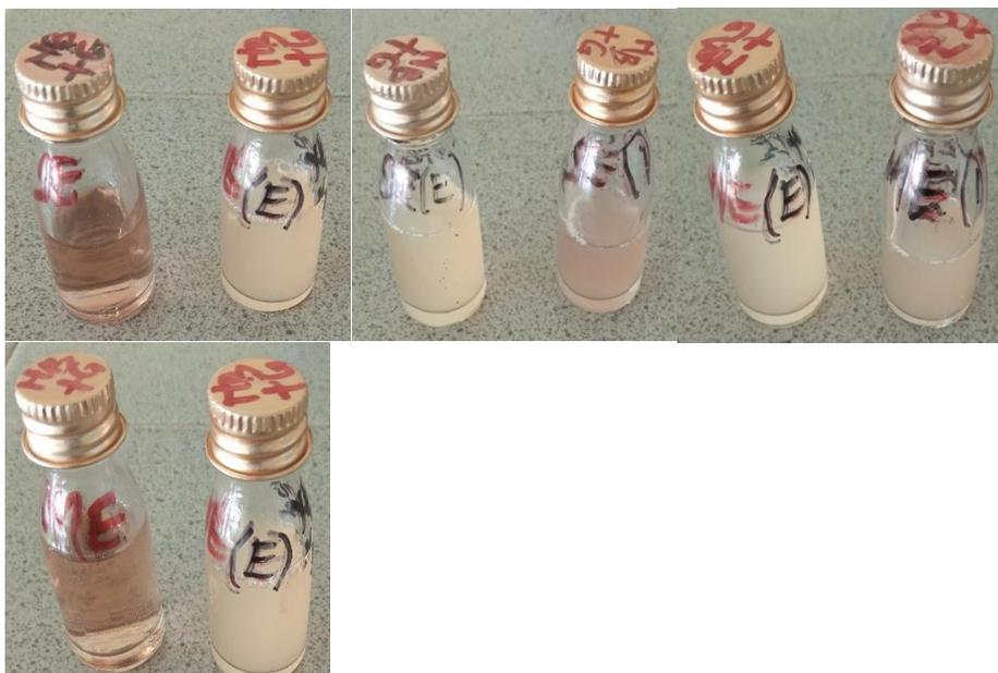
E.2: *Eps* and Isolates Screening for RB5 dye removal with NB+G, GPYMgSO<sub>4</sub> and NB+G broths
