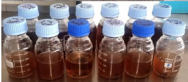
G.2: *Eps*- Bioremediated textile dye wastewater
