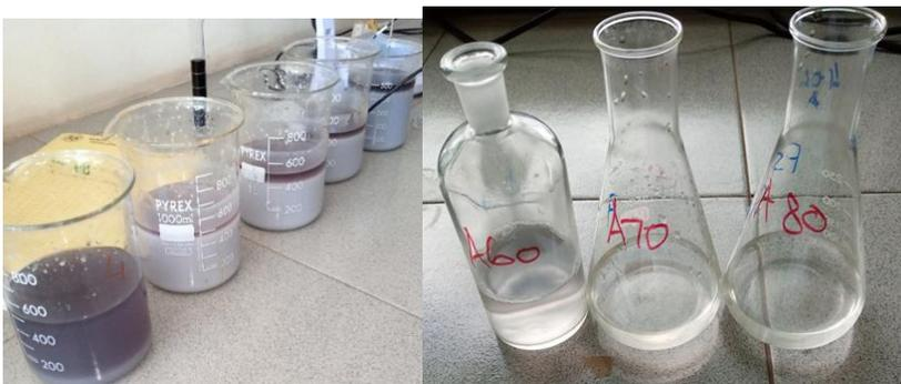
B.1.2: Alum Coagulation of Dye Wastewater- Dosage Optimization
