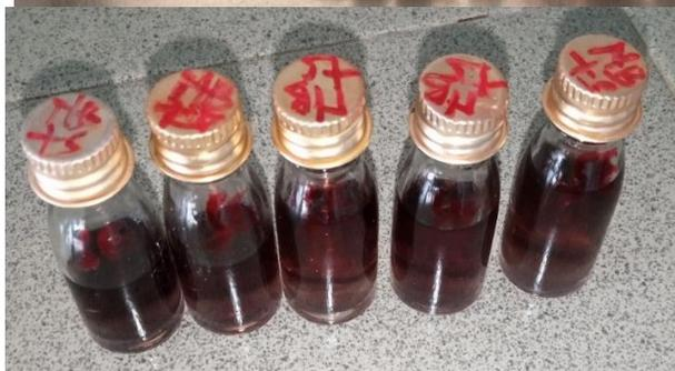
E.1: Machine and synthetic dye wastewater samples inoculated and incubated with *Eps*
