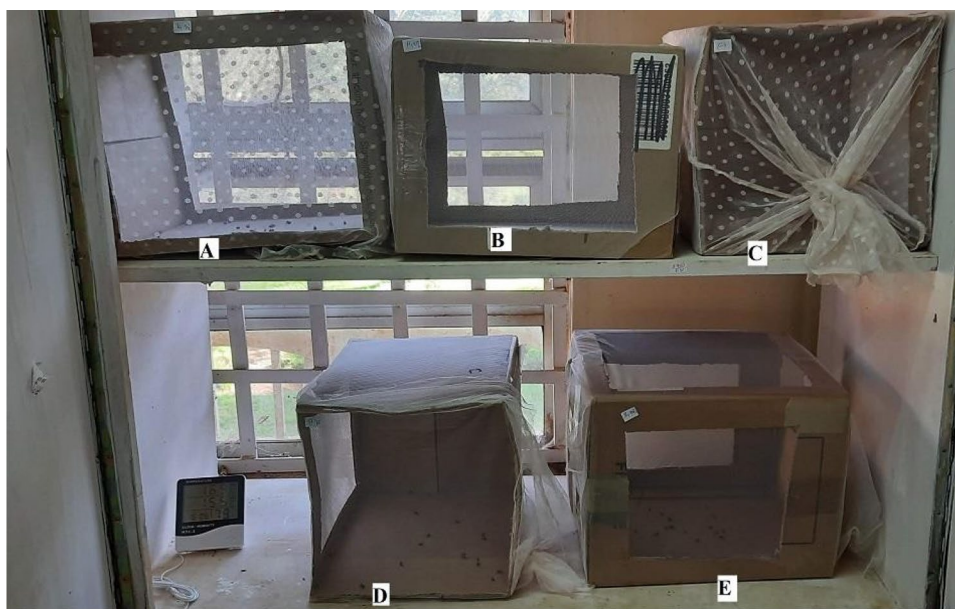
Fig. 3 Bioassay cages for essential oils (A, B and C) and controls (D and E) test experiments (Cage A, B and C were treated with EOs from HLZ, MLZ and LLZ, while D and E was for acetone and DDVP, respectively)
