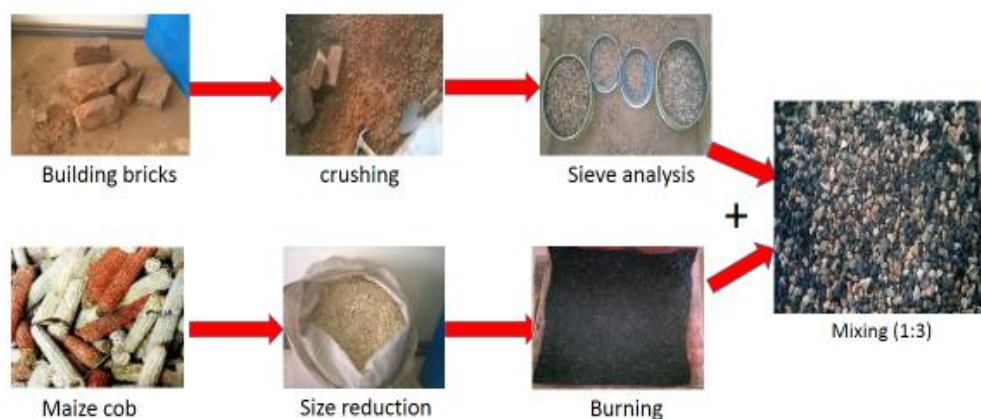
Figure 3.1: Flow diagram for treatment media preparation
