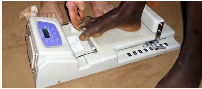
Figure 2: Measurement of hallux flexor strength using the foot strength device.
