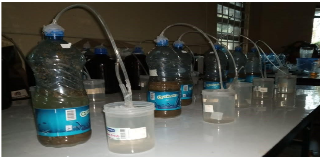
Figure 3.4: Lab-scale setup for co-digestion for different ratios for the 15 days
