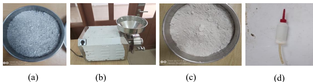
Figure 3.95: Soda ash preparation for adsorption experiment: (a) Large particle size (b) grinder (c) working particle size (d) packed column bed reactor
