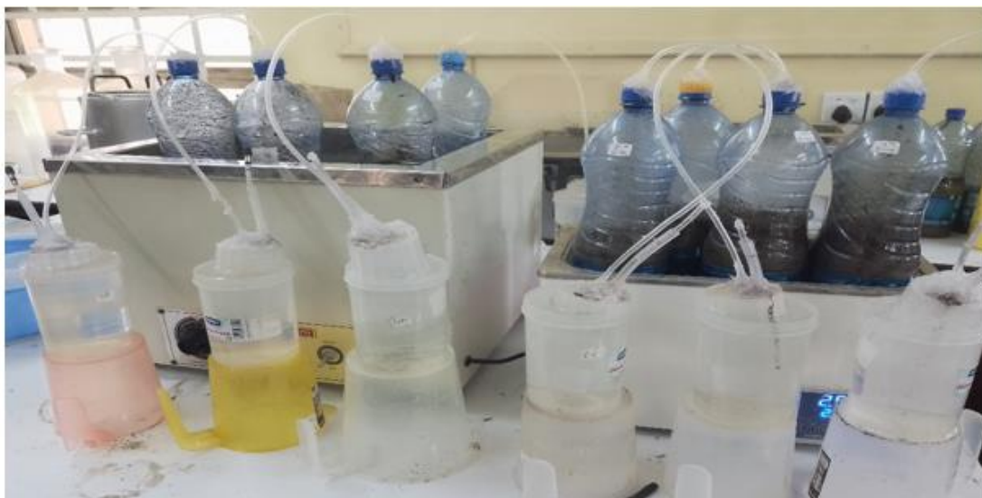
Figure 3.53: Lab-scale setup for co-digestion of TW: FrW on the effect of temperature
