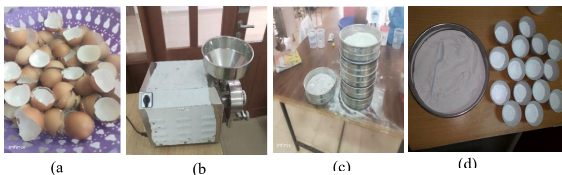
Figure 3.8: Eggshells preparation for adsorption experiment: (a) raw eggshells (b) grinder (c) sieving machines (d) working particle size 280 \mu\text{m}
