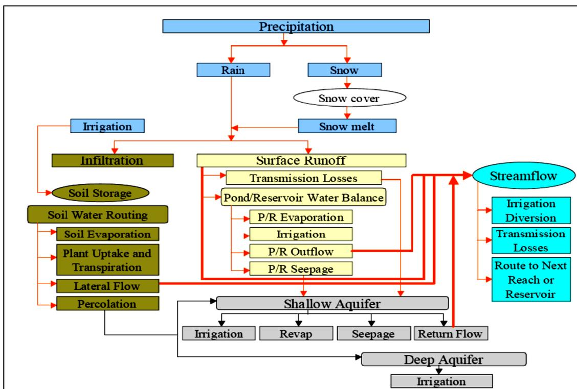
Figure 3.4 Pathways for water movement within SWAT (Neitsch et al., 2004)
