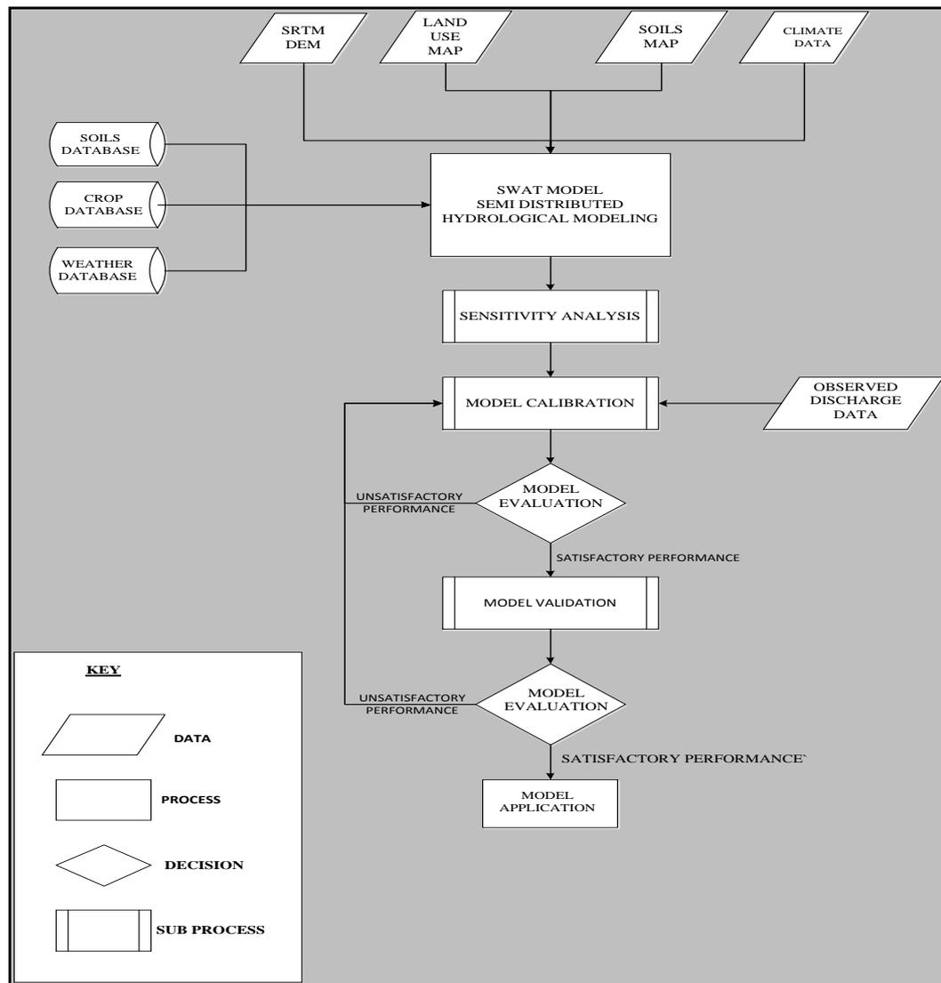
Figure 4.2 Semi Distributed physically based Modelling Approach using SWAT
