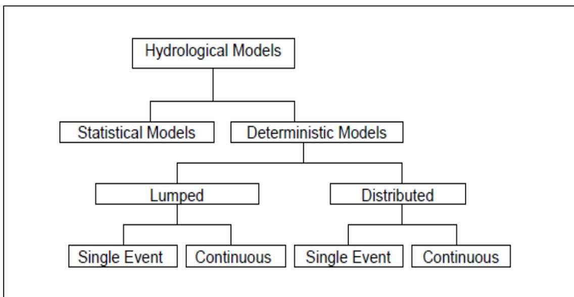
Figure 3.2 Classification of hydrologic models (Bengtson and Padmanabhan, 1999).
