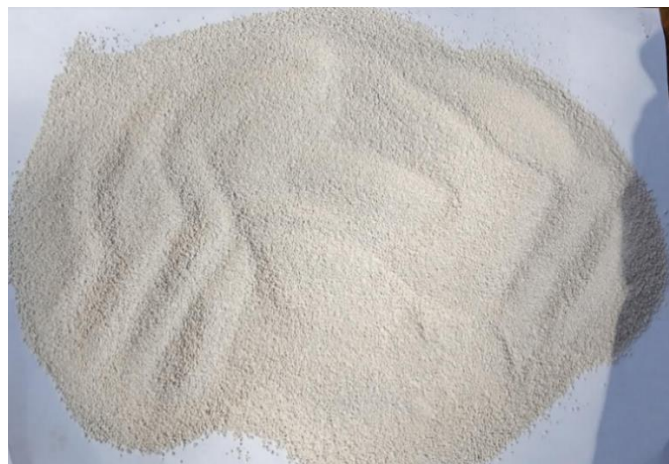
Plate A. 3: Kaolin sieved to 400 \mu\text{m}
