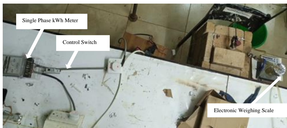
Plate B. 3: Monitoring with Power Meter and Electronic Balance
