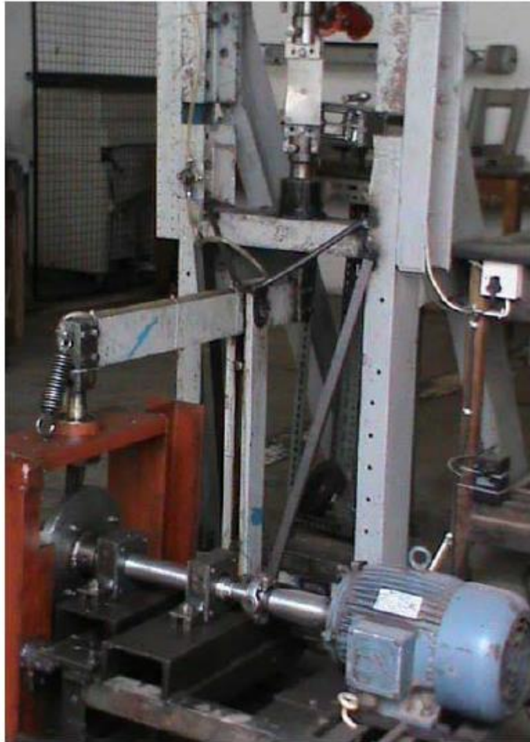
Figure 3.1: Brute force axial-load fatigue testing machine.
