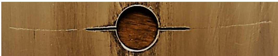
Figure 4.18: Crack path for Al alloy 7075-T7.
