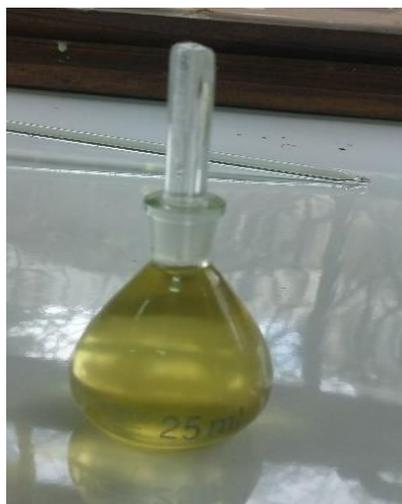
**Figure 3.9: RD Bottle - Specialized container for precise liquid density measurements in scientific investigations.**
