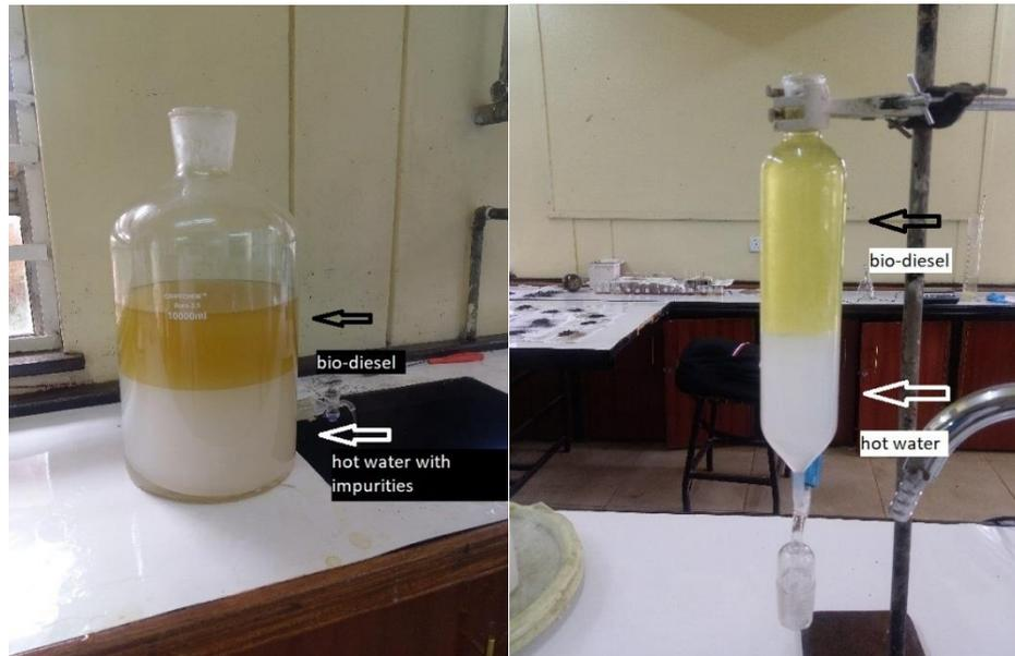
**Figure 3.7: Washing biodiesel in hot water results in a purer end product, highlighting its importance in improving overall synthesis quality.**
