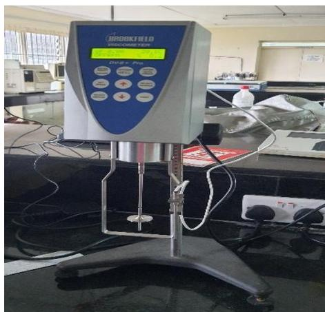
**Figure 3.10: Brookfield Viscometer machine for precise fluid viscosity measurements in scientific and industrial applications.**
