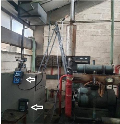
**Figure 3.13: Installed gas detector for measuring emissions in exhaust gases**
