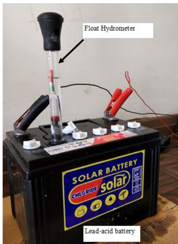
Figure 3.3: Specific gravity measurement using a float hydrometer.
