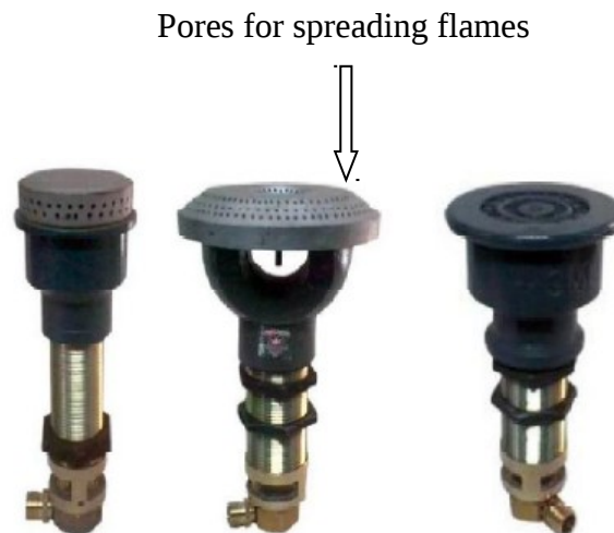
Figure 2.2: Commercial PRB Burners used for Performance Test
