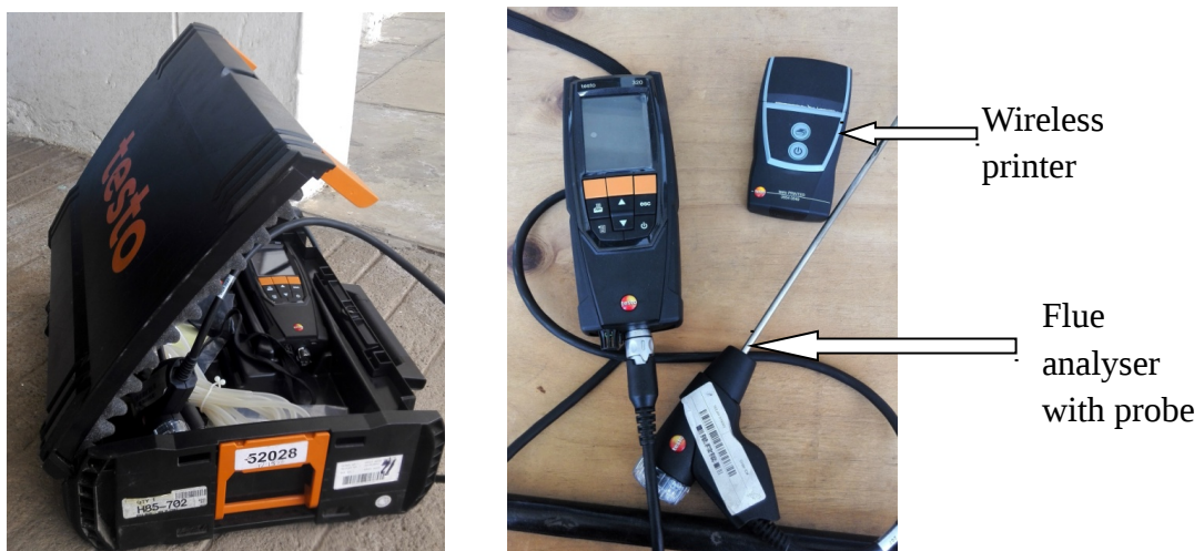
Figure 3.4: TESTO flue gas analyser (Hired from EENONATOTS limited)
