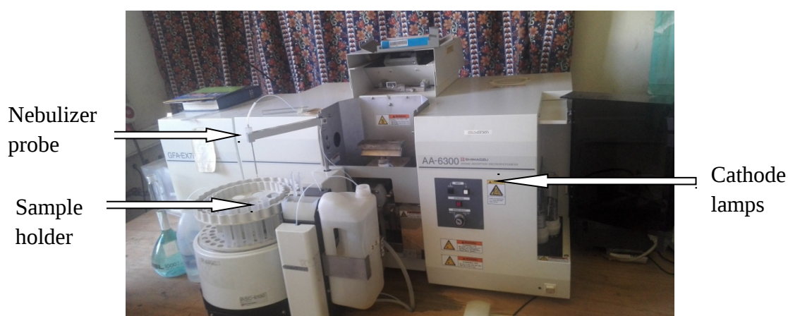
Figure 3.2: Atomic Absorption Spectrometer at KOFC Physiochemical Laboratory
