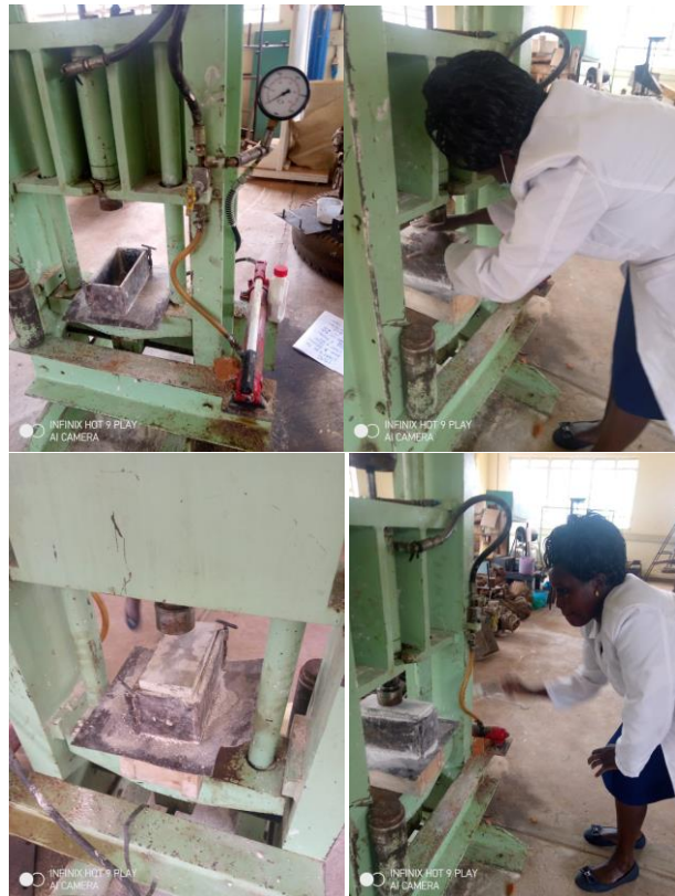
Figure 3.8: Moulding and compaction process
