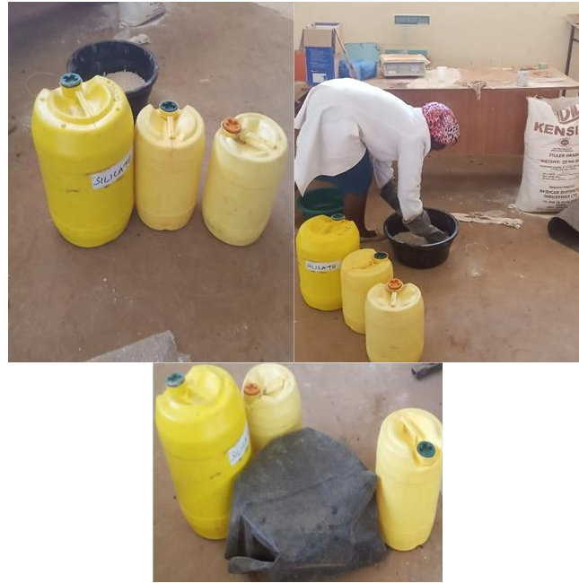
Figure 3.10: NaOH/Na 2 SiO 3 activated geopolymer preparation
