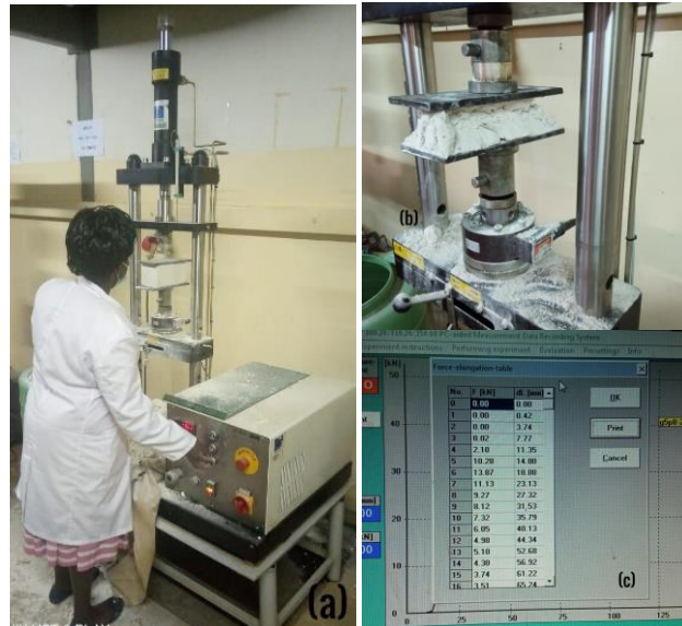
Figure 3.14: Compression strength testing process
