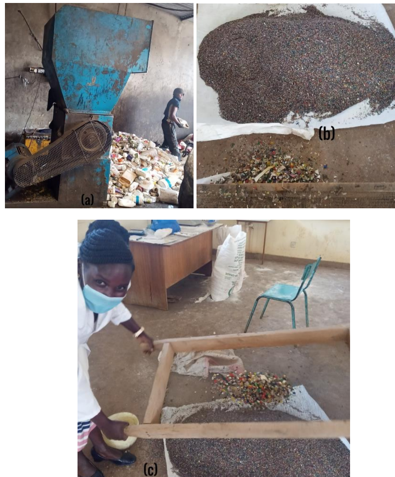
Figure 3.5: HDPE Preparation (a) Shredding (b) Drying (c) Sieving
