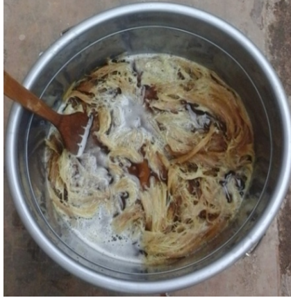
Figure 12: Surface treatment of pseudo-stem banana and sisal fibres
