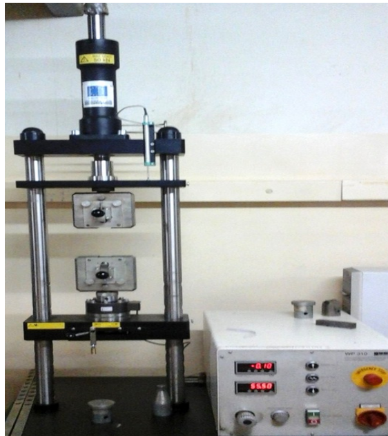
Figure 15: Universal material tester used for banana and sisal bio-composites tests
