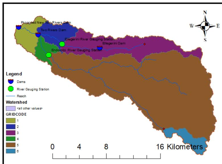
Figure 4.2 Two Rivers Dam catchment Sub Basins
