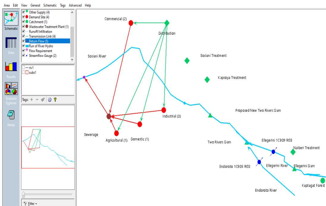
Figure 4.20 Schematic presentation of the Two Rivers Dam catchment system and demands in WEAP
