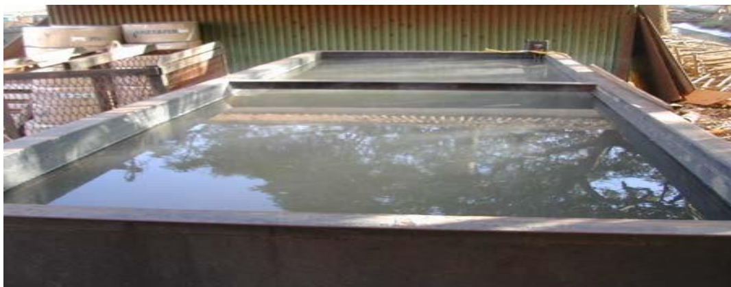
Figure D3: Leaching tank
