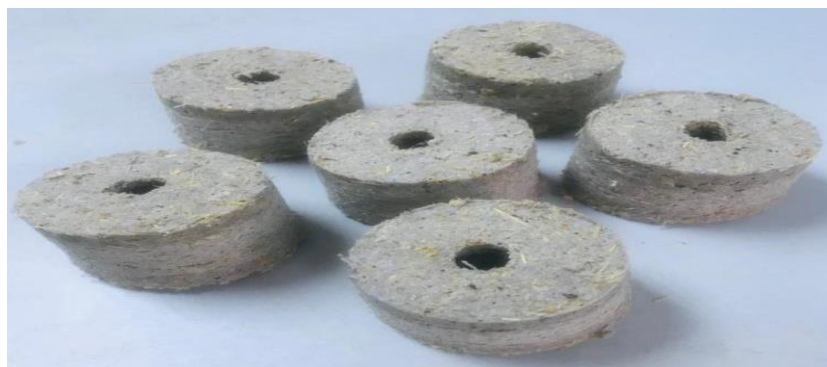
Figure 2.4: An example of briquette made using a manual piston press (Wu et al, 2019)
