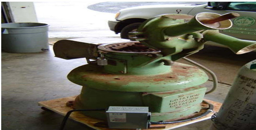
Figure. D1: Jeffco Cutter Grinder (Jeffress Bros. Ltd, Queensland Australia) used for particle size reduction of cane trash samples.
