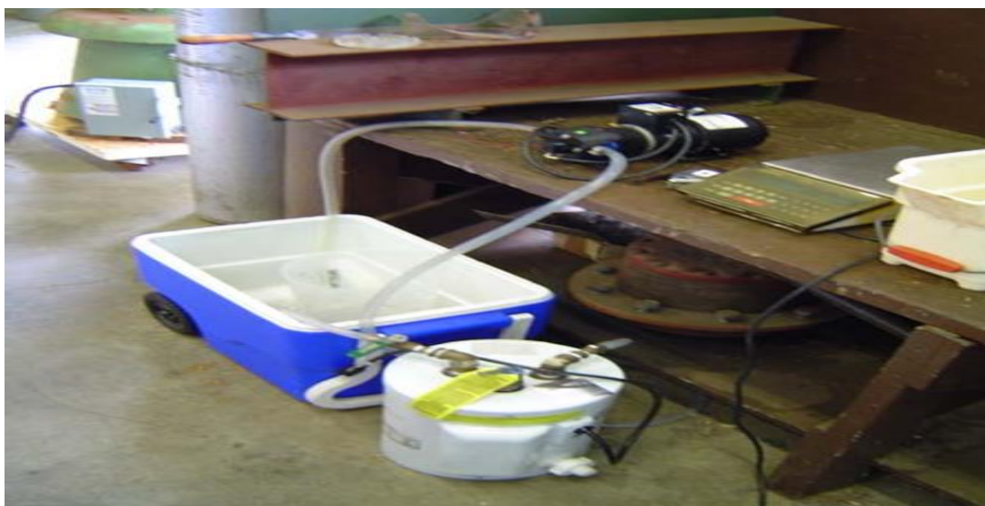
Figure D2: Heating bath, heater and pump used to maintain temperature during "Hot" laboratory scale experiments
