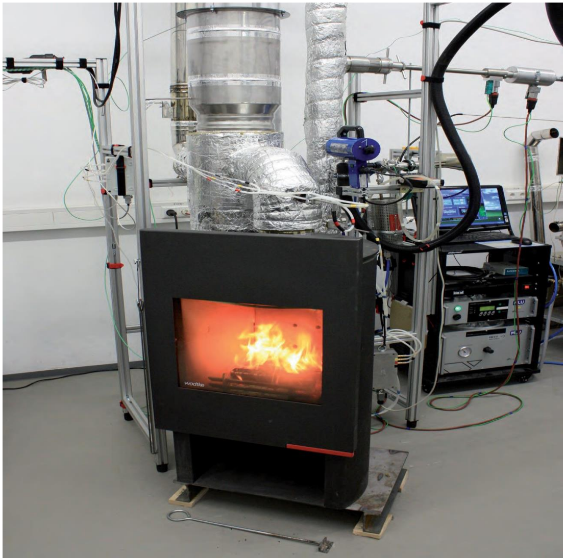
Figure D8: Combustion analysis system set up
